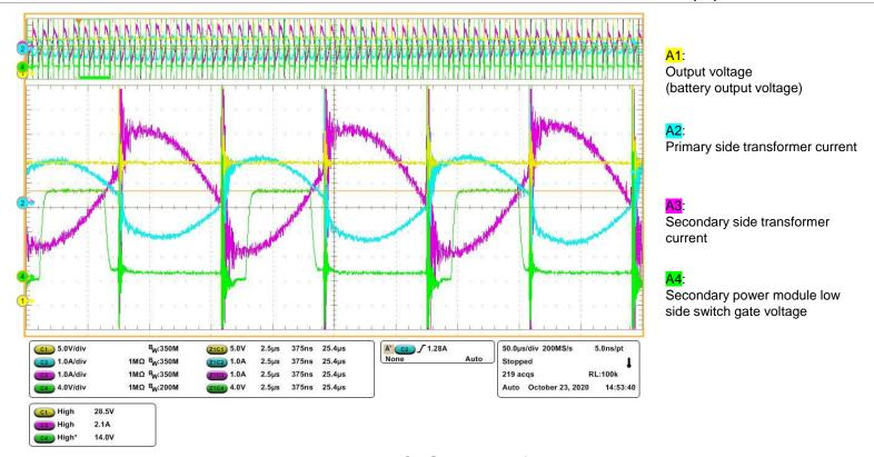
Input voltage 60  $V_{DC}$ ,  $R_{LOAD}$  23,5  $\Omega$ , Switching frequency 120 kHz
