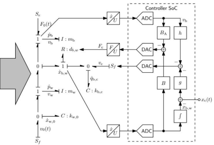
Equivalent representation using bond graphs for the energy conservation part and block diagrams for the signal processing part
